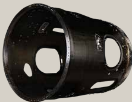
OUTER BYPASS DUCT
